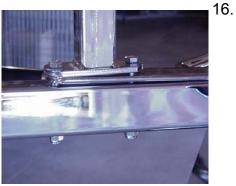
Connect the hip flexor weldment to the diagonal bar (Item 6) directly above. Sandwich the mounting plate weldment from Step 15 between the plate end of the side mounted hip flexor weldment (Item 166) and the hip flexor weldment, using screws (Item 53) and nuts (Item 4) to make the attachment. Use screws (Item 59) and nuts (Item 4) for the upper connection to the diagonal bar.
