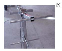
Insert the two roller shafts (Item 172) through the T/K arm (Item 175) and secure each shaft using a screw (Item 135) and locking washer (Item 60). Assemble two rollers (Item 78) to each roller shaft. Use the following sequence for each: one aluminum disk (Item 58), one nylon washer (Item 177), a roller, one nylon washer (Item 177), one aluminum disk (Item 58), and a retaining ring (Item 171). Follow the instructions provided with the upholstery pack for proper assembly of the retaining rings.
