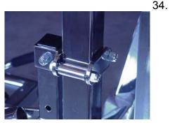
Attach the top of the adjust tube to the frame post. Slip the top bracket (Item 2) down over the top of the tube and attach using a screw (Item 5) and locking nut (Item 3). Locate the two spacer tubes (Item 35) and mounting tab (Item 4). Use two screws (Item 34) and locking nuts (Item 3), along with the spacers and tab, to attach the top bracket to the frame post. Tighten all hardware assembled to this point.
