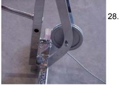
Locate the T/K short cable assembly (Item 183). Lay the cable assembly in the T/K leg (Item 178) with the hook toward the main frame. The cable will lie across a pin welded near the bottom of the leg. Assemble a pulley wheel (Item 143) into the T/K leg using a screw (Item 170) and locking nut (Item 67). Be sure that the cable is in the groove of the pulley wheel.
