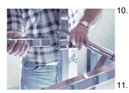
Install the **Shoulder Press** arm assembly (**Item 102**). With the handle angle towards the floor, slide the tube portion through the DVR bracket at the top of the weight stack and attach it to the pivot tube (**Item 103**) tabs at the opposite end of the main frame. Secure using screws (**Item 59**) and locking nuts (**Item 4**).
