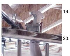
19. Attach the upper fixed pulley bracket (Item 144) to the top of the top frame between the low pulley runner guides. Use two screws (Item 53) and locking nuts (Item 4).
