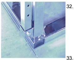
32. Assemble the square plastic plugs (Item 14) to the adjustable upright tube (Item 17). Stand facing the side of the unit that the bottom bracket is on. Insert one end of the upright tube down into the bracket, making sure that the adjust holes of the upright are to the right side. Loosely assemble using a screw (Item 5) and locking nut (Item 3).
