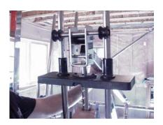
5. Install the **Leg Press** station weight stack next to the Shoulder Press stack.
